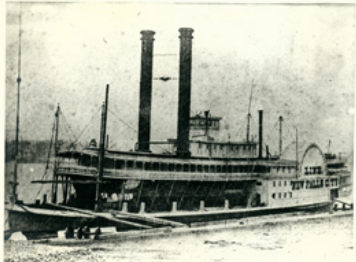
Built in 1850; hull 231'x45'x7 1/2'; DR; 6 boilers, 40" x 28"; cyl. 30"X30"; sunk in Red River above Springfield Landing in 1864 to prevent passage of Porter's fleet.
