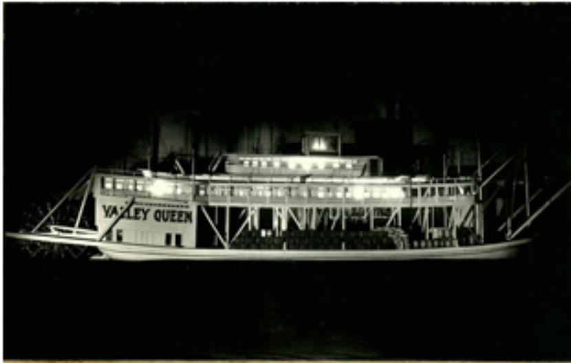
Model of the Red River line Steamer VALLEY QUEEN - 1/2 in. scale. Built in 1899 at Jeffersonville, Ind. Hull, 196 X 36 X 6 ft. Ran in Red River trade and Saint Louis-New Orleans trade under charter of Anchor Line, S. C. Lee, Master. Model built by E. Phillip Norman of New York City in 1933-34. This photo shows model in a "right" aspect all "left" on.
